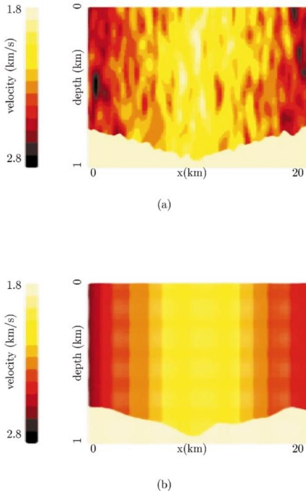
FIG. 8. (a) True synthetic velocity model (horizontal gradient, Gaussian covariance,  $\sigma_\epsilon=4\%$ ,  $a=0.4 \text{ km}$ ,  $b=0.1 \text{ km}$ ,  $\Lambda=4$ ) and reflector (gradient, Gaussian covariance fluctuations,  $\ell_\eta=0.4 \text{ km}$ ). (b) Inverted velocity model by traveltimes tomography.
