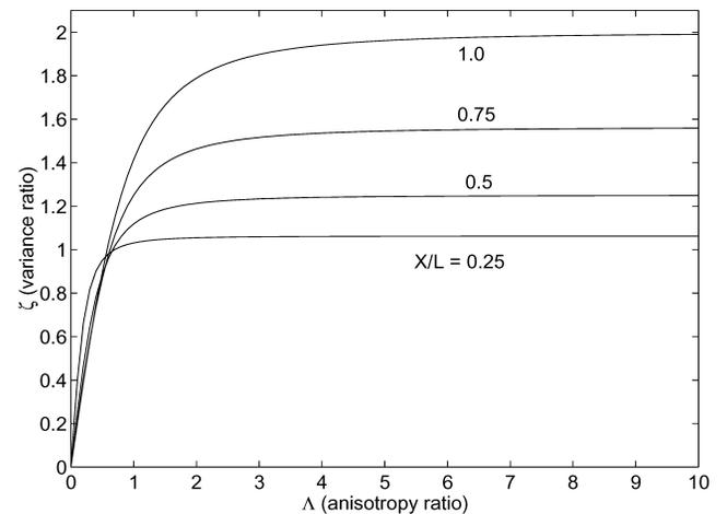
FIG. 4. Traveltime variances ratio  $\zeta = \text{var}T(X, L)/\text{var}T(0, L)$  as a function of  $\Lambda$  [equation (19)], for different values of  $X/L$ .
