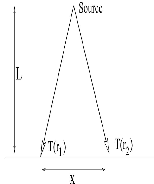
FIG. 3. Geometry of two straight rays leaving a point source. Traveltimes  $T(\mathbf{r}_1)$  and  $T(\mathbf{r}_2)$  are measured at a vertical distance  $L$  from the source and are laterally separated by a distance  $x$ .
