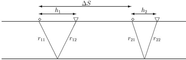
FIG. C-1. Scheme of the lay-out:  $\Delta S$  is the distance between two sources;  $h_1$  and  $h_2$  are two offsets;  $r_{11}$  and  $r_{21}$  are the downgoing rays while  $r_{12}$  and  $r_{22}$  are the upgoing rays.
