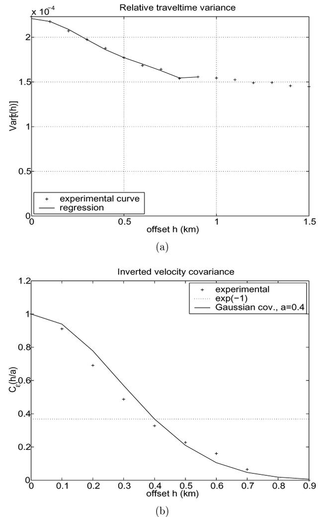
FIG. 9. (a) Experimental relative traveltimes variance as a function of the offset corresponding to the model in Figure 8a. The polynomial fit is calculated by least-squares regression. (b) Inverted velocity covariance by prestack statistical tomography. Comparison is made with the true velocity covariance (Gaussian curve).
