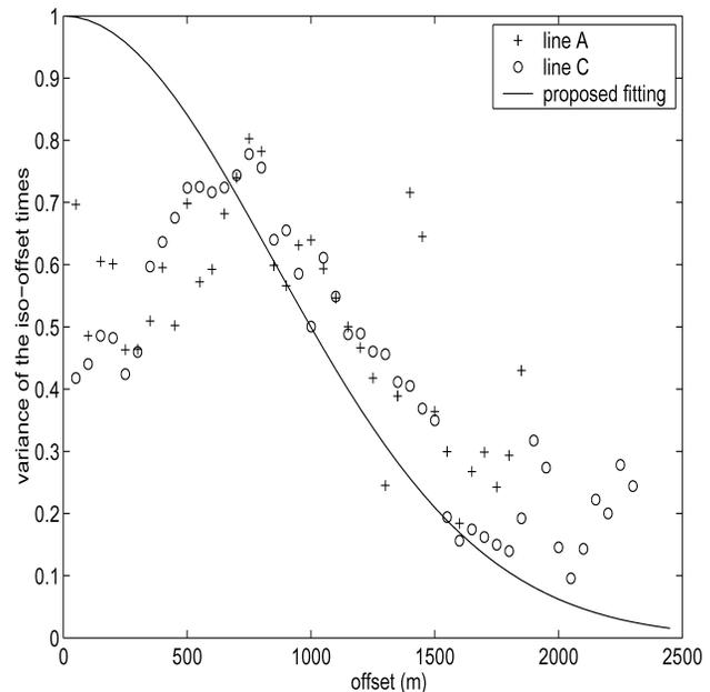
FIG. 12. Normalized variance of the iso-offset traveltime collections for acquisition lines A and C. The proposed curve fit is calculated with  $a = 1200$  m for the horizontal correlation length of the velocity field.
