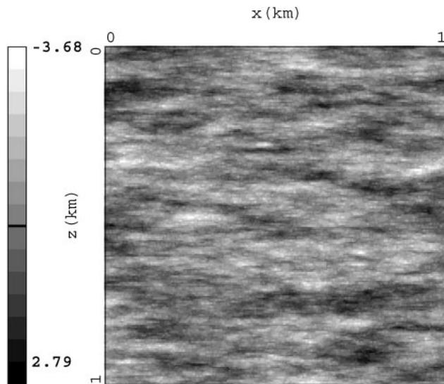
FIG. 1. One realization of a 2D anisotropic random perturbation with an exponential covariance, a variance  $\sigma^2 = 1$ , a horizontal correlation length  $a = 0.1$  km, a vertical correlation length  $b = 0.02$ , which leads to an anisotropy ratio  $\Lambda = a/b = 5$ .
