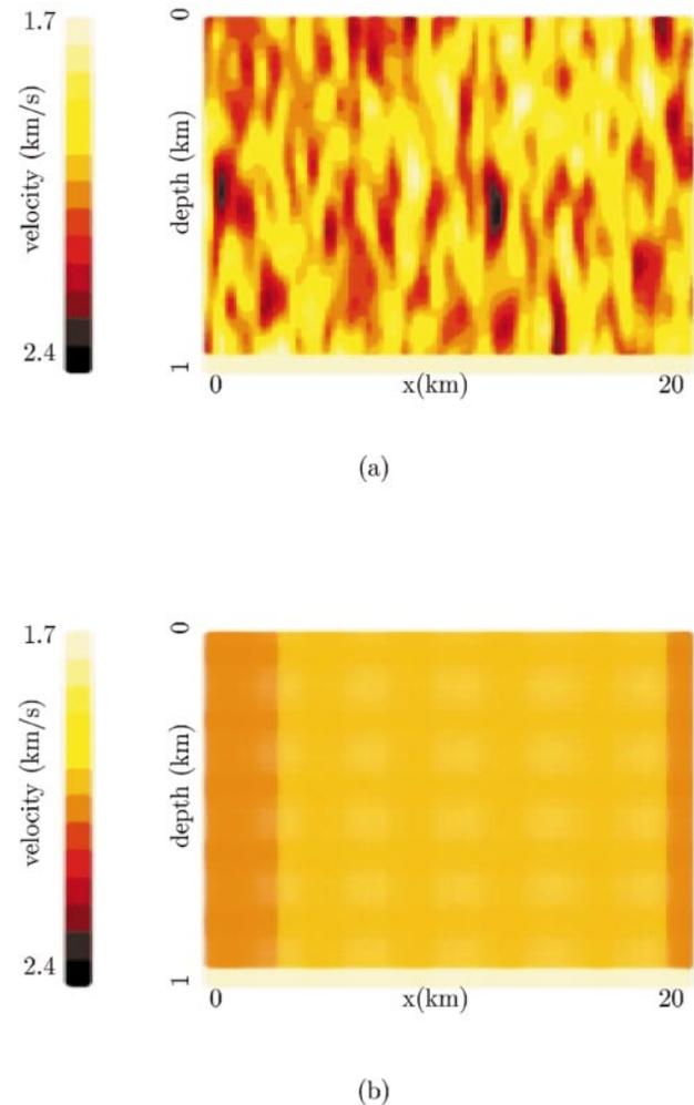
FIG. 5. (a) True synthetic velocity model (Gaussian covariance,  $\sigma_\epsilon = 4\%$ ,  $a = 0.4$  km,  $b = 0.1$  km,  $\Lambda = 4$ ) with horizontal reflector. (b) Inverted velocity model by traveltime tomography.
