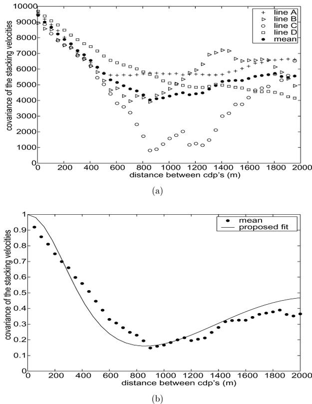
FIG. 13. (a) Stacking velocity covariances [in  $(\text{m/s})^2$ ] for the four different lines and the calculated mean. (b) Mean normalized covariance of the stacking velocities and its proposed fit.
