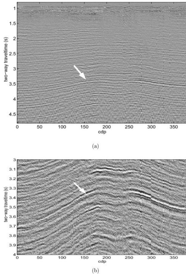
FIG. 11. (a) Prestack seismic section (offset  $x = 350$  m) in the time domain (in seconds). The white arrow shows the picked reflector. (b) Zoom on the picked reflector (in seconds).
